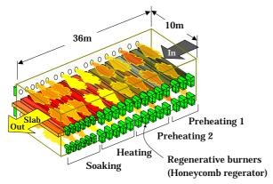
Fig.5 Regerative burner type reheating furnace
