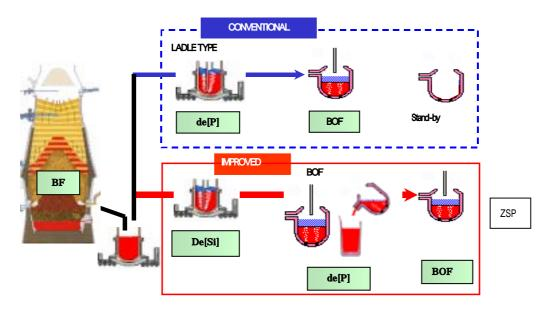
Fig.2 ZSP (Zero Slag Process) at Keihin Works
